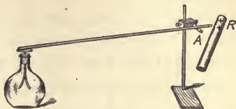
FIG. 275.—Testing the Conductivity of Rods.
